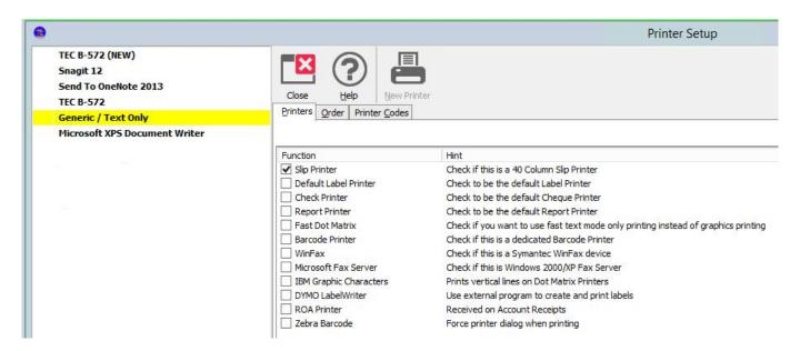
Cutting of receipts is also controlled from the Windows printer driver. It is also recommended that you do not use the Generic Text Driver in Windows. Use the correct driver for your printer to ensure that the cutter and cash drawer settings are correct for your specific printer.
